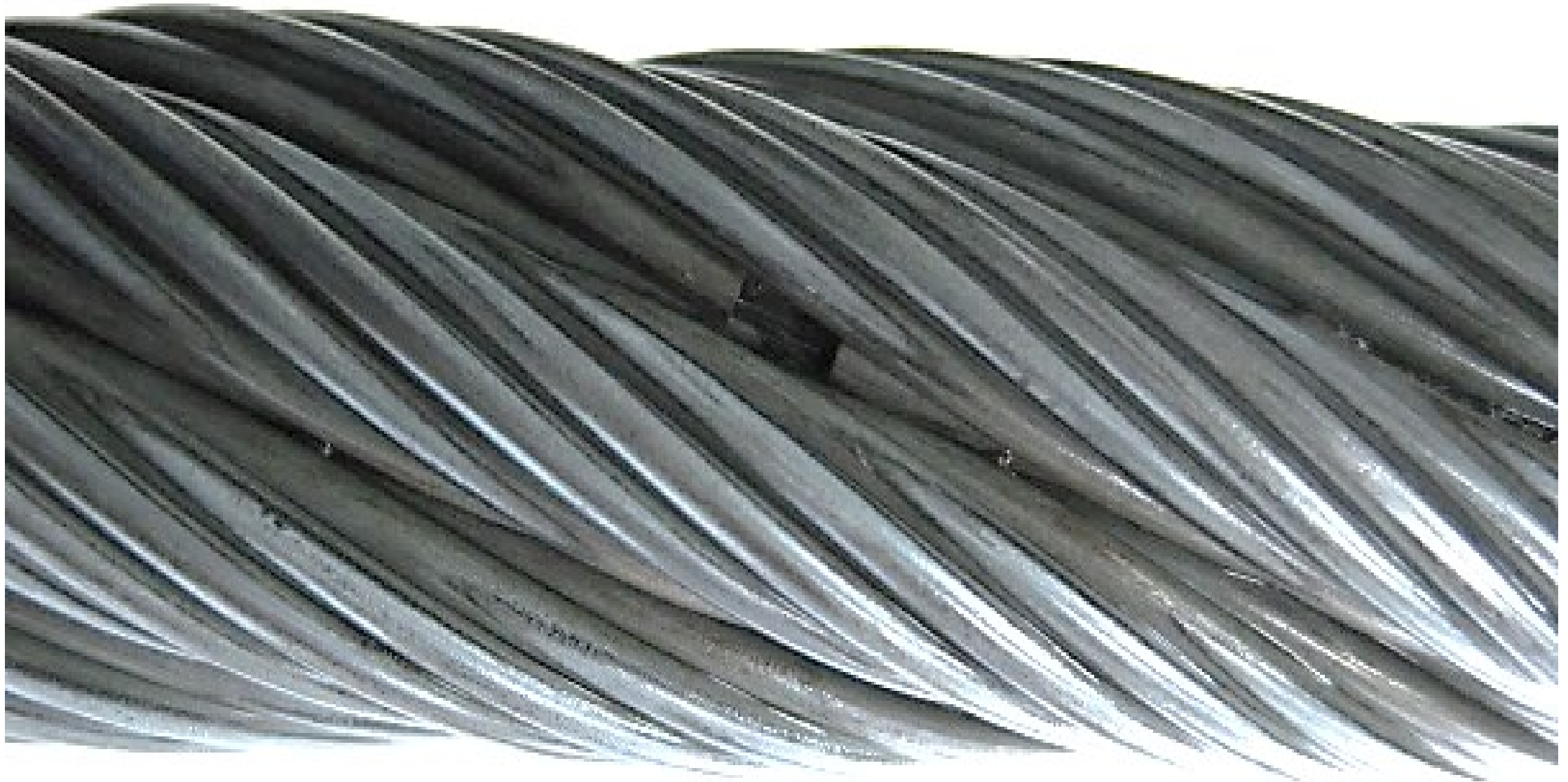
Common wire break due to bending cycles
