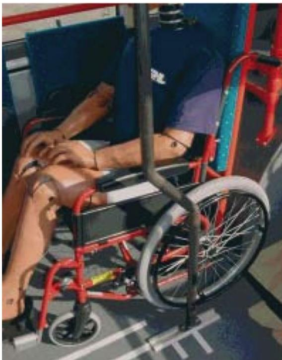
**Figure 35** Wheelchair space fitted with stanchion
