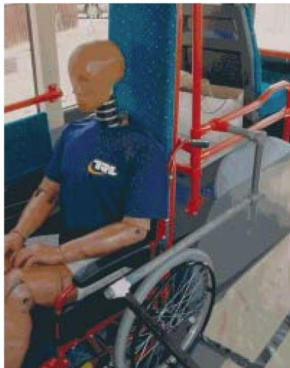
**Figure 36** Wheelchair space fitted with rail
